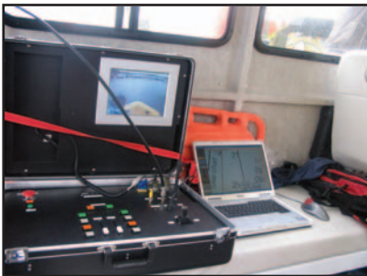
Left to right: This high-tech security control terminal aboard the USV can be operated manually, or via remote control for many different types of missions. • A laptop computer is a key part of the USV terminal station. • An omnidirectional antenna and video cameras are perched atop the USV. • This Global Positioning System (GPS) antenna and receiver relay are key elements of the USV's control system.
