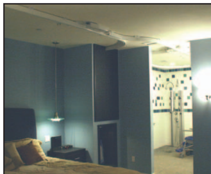
Supported by the strength of extruded aluminum, the ceiling track lift system gives Rodney Anderson newfound mobility, transferring him from bed to bathroom to wheelchair with ease.
