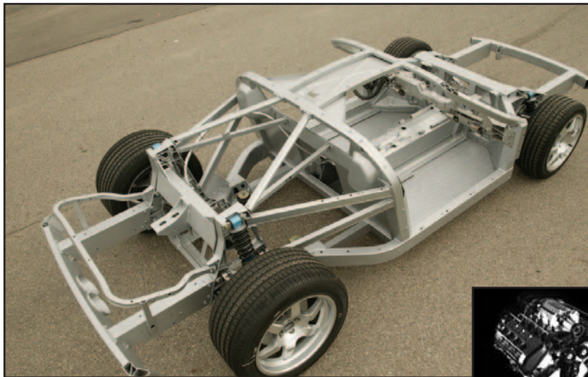
GT's extruded aluminum space frame makes automotive design history.
