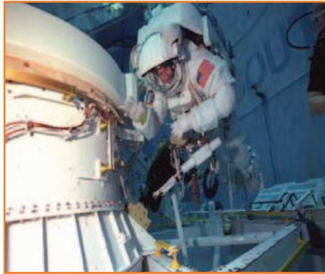
*An astronaut wears a training version of the extravehicular mobility unit (EMU) space suit during an underwater simulation of a space walk, conducted in the Neutral Buoyancy Laboratory in Houston, Texas.*
