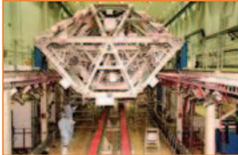
*Truss segment Starboard Zero (SO) takes center stage. Workers check the structure, as the Canadian Mobile Transporter, power distribution system modules, heat pipe radiator for cooling, and a pair of rate gyroscopes are installed. The structure will ultimately extend the length of a football field.*
