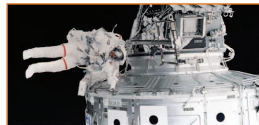
*Hanging tough: During space walks, astronauts rely on every extruded aluminum handrail to do its job without fail. Handrails are always within reach, serving as tether anchors for equipment, and lifelines for the ISS crew.*
