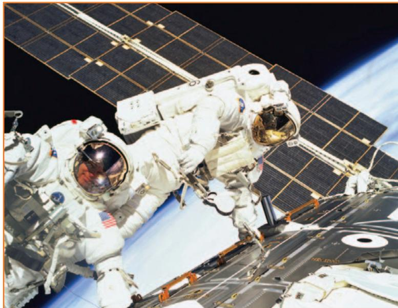
crewmember on an EVA. Critical to all EVAs are the hundreds of extruded aluminum handrails covering the exterior of the International Space Station, which allow the astronauts to negotiate the vast truss structures during construction assemblies. Handrails are also used to tether lines that attach to crew and equipment for tests and repairs that occur round the clock, 365 days a year. Each handrail is distanced apart from the next one by the length of an astronaut's reach.
